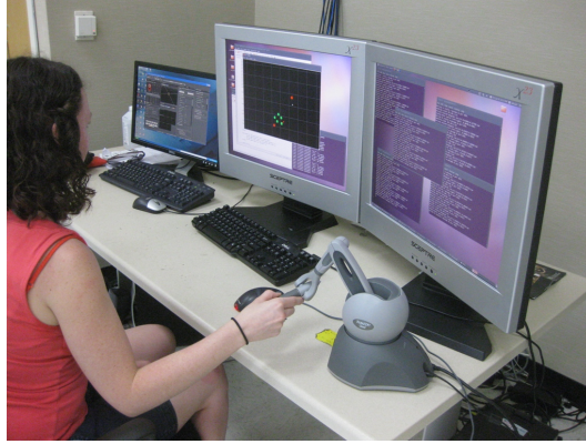
Figure 3. Photo of student utilizing haptic device while looking at the virtual environment (middle screen).
