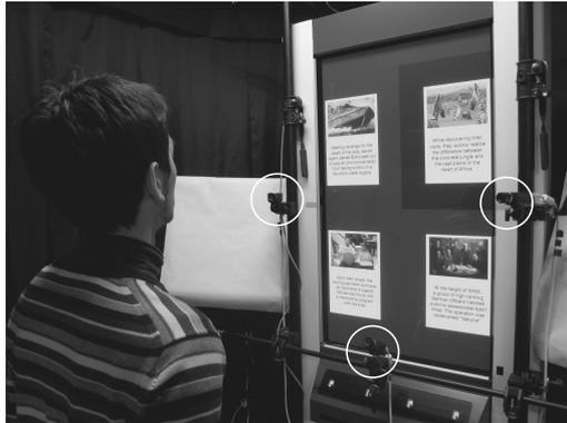
**Fig. 1** Prototype information service system with a large display and three cameras (circled in white).
